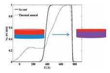
Fullerene diffuses into low-bandgap polymers with thermal annealing. Polymer/ fullerene mixing is found to be crucial for optimal device performance.
