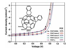
The trans-2, trans-3, trans-4, and e isomers of dihydronaphthyl-based [60] fullerene bisadduct (NCBA) are isolated and used as acceptors for P3HT-based polymer solar cells (PSCs), and the corresponding PSCs fabricated by the four isomers show power conversion efficiencies of 5.8, 6.3, 5.6, and 5.5%, respectively, which are higher than that based on an NCBA mixture (5.3%), suggesting the necessity to use the individual fullerene bisadduct isomer for high-performance PSCs.
