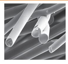
A novel synthetic technique for lignin-based carbon fibers, where the fibers are fused to each other resulting in monolithic fibrous mats, is described. The unique fiber microstructures and mat morphologies provide favorable electrochemical performance for lithium ion battery anode applications. The fibers cycle reversibly versus Li metal in alkyl carbonate electrolytes.
