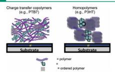
The excitonic dissociation pathways in the high-performance, low bandgap "inchain donor-acceptor" polymer PTB7 are investigated by transient absorption spectroscopy and grazing incidence spectroscopy. The effects of the amplitude and kinetics of inter- and intramolecular charge transfer state spectra, along with a detailed morphology analysis, are investigated and compared to those of conventional semiconducting homopolymers.
