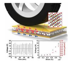
The unidirectional high-power generation via stress-induced dipole alignment from single-crystalline piezoelectric perovskite ZnSnO $_3$  nanocubes/polydimethylsiloxane hybrid piezoelectric nanogenerator without applying electrical poling is demonstrated. A recordable large output voltage of about 20 V and an output current density value of about 1  $\mu$ A cm $^{-2}$  from a single nanogenerator cell are successfully obtained under rolling of a vehicle tire.
