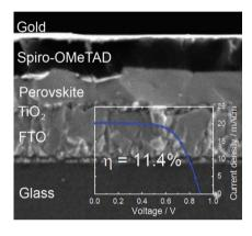
The critical role of perovskite morphology in planar heterojunction perovskite solar cells is probed and understood. Dewetting of perovskite films is minimized, to achieve uniform 100% coverage perovskite layers. Solution cast planar heterojunction solar cells with efficiencies of up to 11.4% are fabricated, a new record for such cells with no mesoporous layer.
